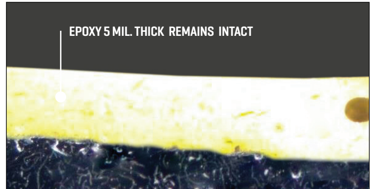
After Temperature Cycling Test: NewAge's epoxy coating remains intact with minimal evidence of wear, which promotes performance longevity and extended service.
